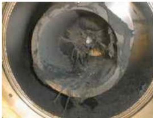
Photograph of the inner chamber of an experimental arc-discharge reactor
